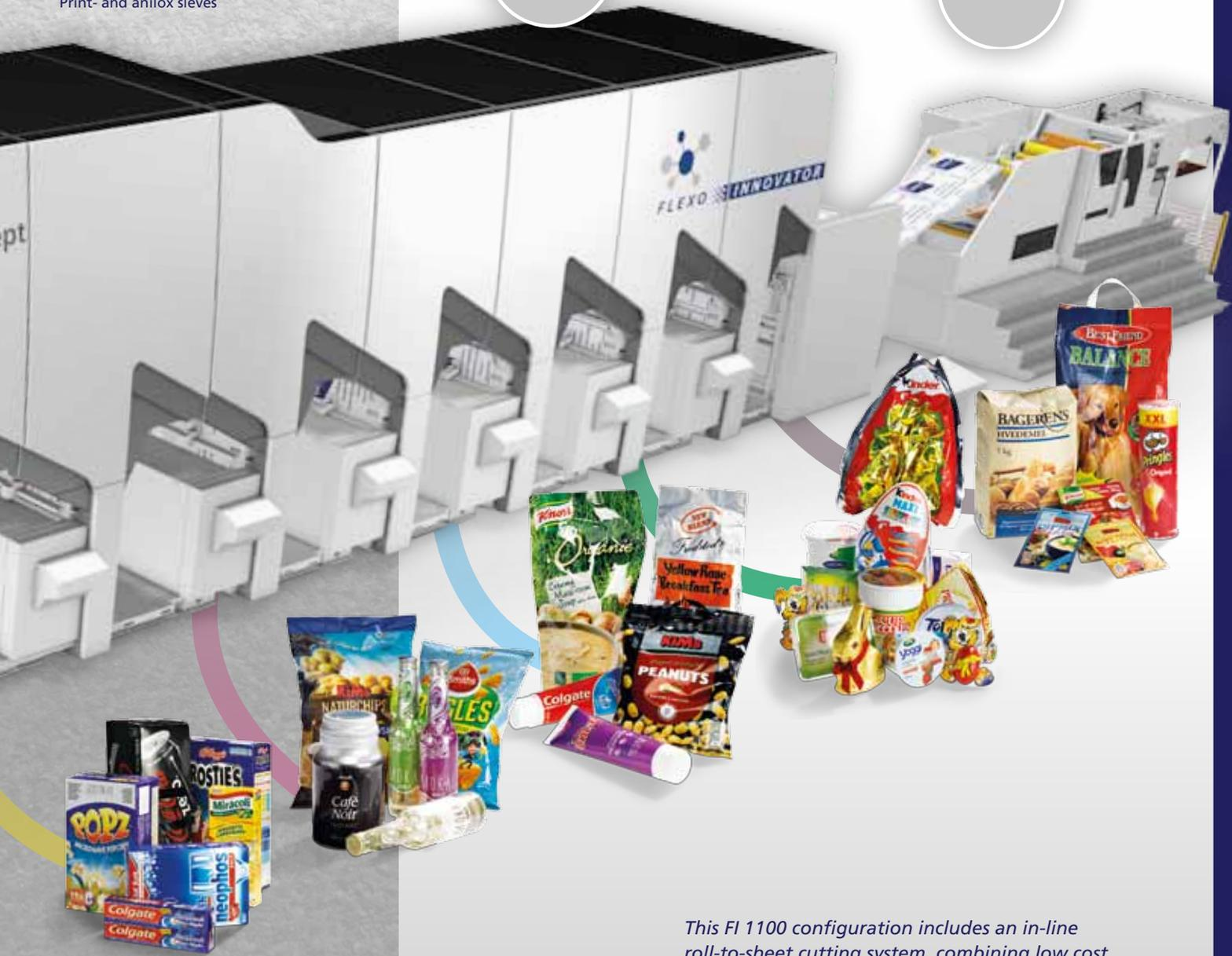
*This FI 1100 configuration includes an in-line roll-to-sheet cutting system, combining low cost of ownership with high productivity.*
