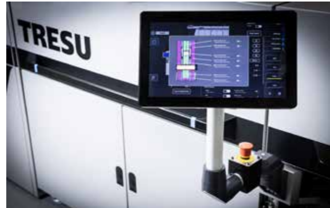
Fast set-up and easy job changes with HMI recipe storage: Complex job details recalled at the push of one button. (PLC included).
