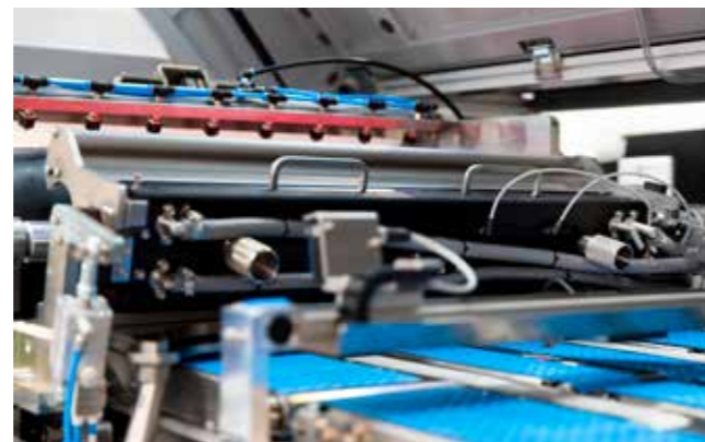
Genuine TRESU chamber doctor blade system designed for fast handling and great performance.
