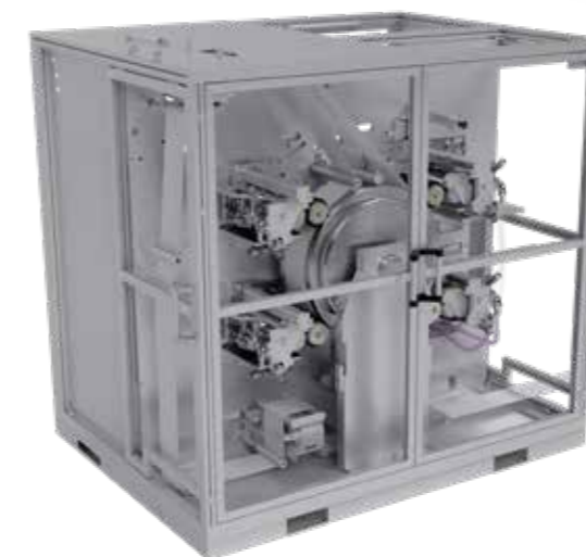
TRESU CI Inline Flexo C4 - up to 4 print units
