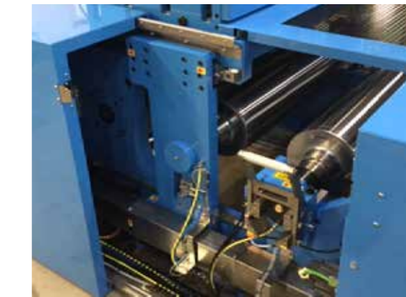
Retrofit flexo adhesives unit 1000 m/min
