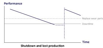
Replacing wear parts when needed will save you from unnecessary downtime and service based on costly and timeconsuming assumptions.
