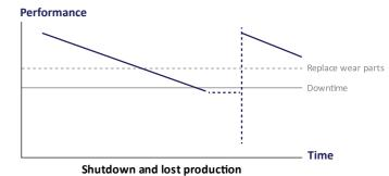
Replacing wear parts when needed will save you from unnecessary downtime and service based on costly and timeconsuming assumptions.
