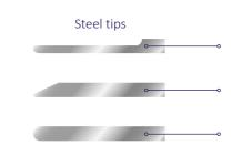
**Lamella** Lamella profiles are used in coating but also gravure and flexo printing. A lamella profile wipes well, up to the point that the contact zone becomes too large. They are available in different angles - pls. inquire for more details.
