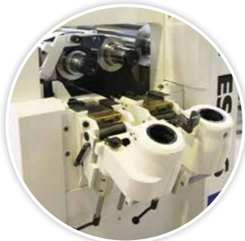
Plate and Anilox Rollers Sturdy construction with tilted roller bearings on the operator side for easy change of plate and anilox rollers.
