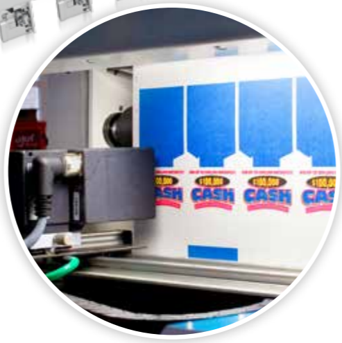
Register Control Fully automatic traverse. Eltromat register control system with complete, automatic pre-setting ability.
