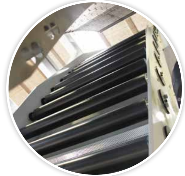
Hot-Air Drying System The hot-air drying system achieves air speeds of up to 65 m/min – thus preventing web shrinking. Automatic regulations means that approx. 15-25% of the air is constantly renewed. The system provides easy web access for cleaning and comfort, great colour consistency and very few recirculation losses.
