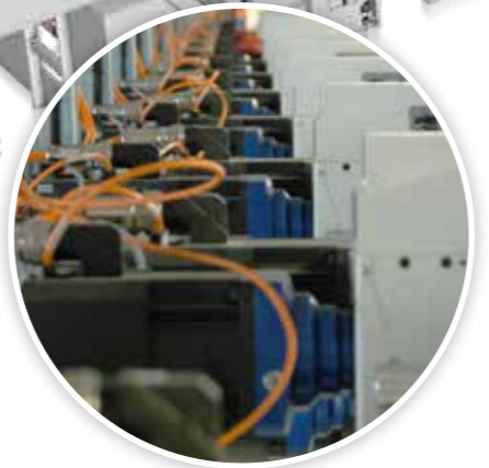
Full Electronic Drive Each print unit is equipped with eight servo motors – for the anilox roller, the plate-, and the impression cylinder.
