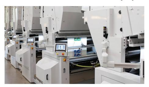
To accelerate setup times further, packaging converters commonly prefer eight to ten printing stations, even though the majority of jobs are seven colours or fewer. In most cases, therefore, the operator can prepare the next job's idle stations while the previous job is in production, thereby cutting waiting times.
